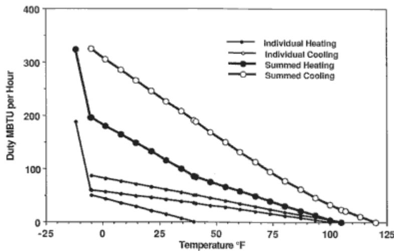
Figure 5. Incremental duties for complex exchanger for liquids recovery unit in Case 1.
