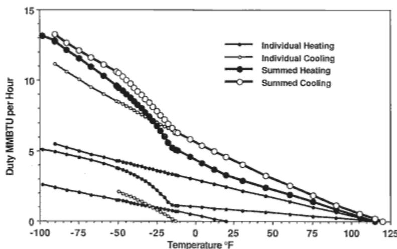
Figure 9. Final trial: Incremental duties for complex exchanger for ethane recovery unit in Case 2.
