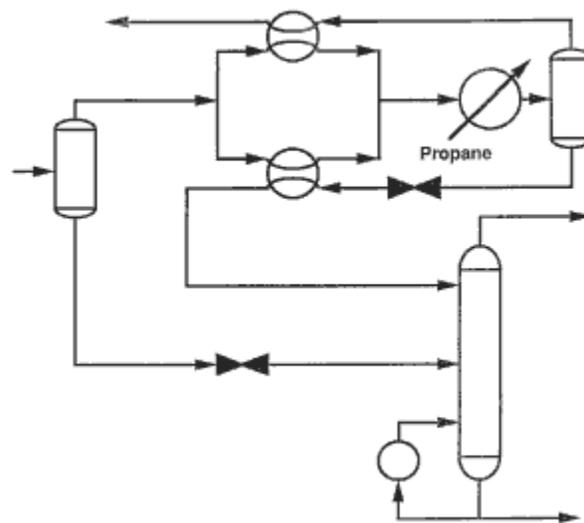
Figure 2. Liquids recovery unit with conventional exchangers for Case 1.
