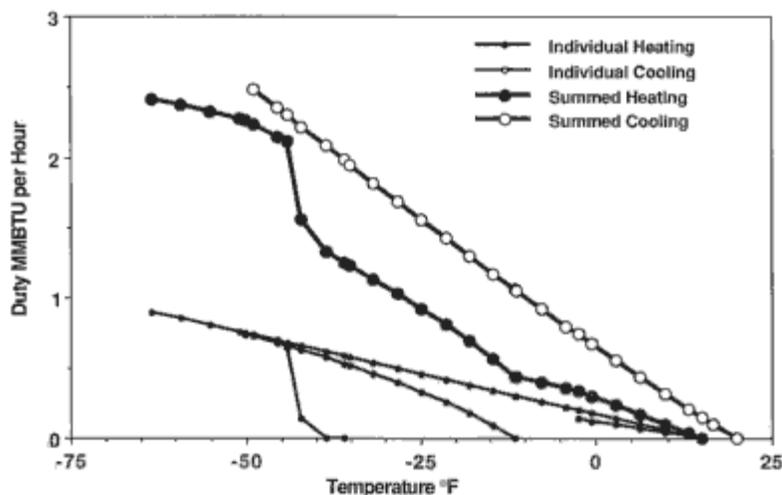
Figure 12. Incremental duties for second complex exchanger for liquids recovery plant in Case 3.
