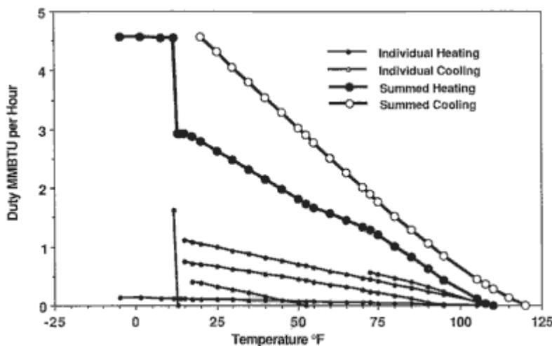
Figure 11. Incremental duties for main complex exchanger for liquids recovery plant in Case 3.
