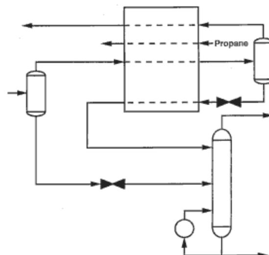
Figure 3. Liquids recovery unit with complex plate exchanger for Case 1.
