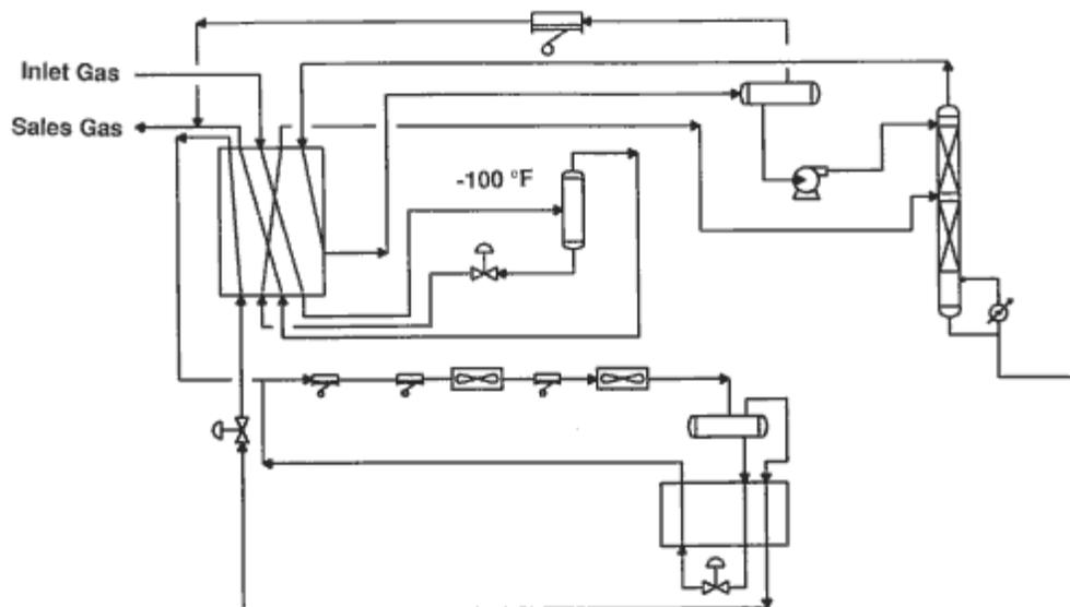
Figure 6. Process flow for ethane recovery using mixed refrigerant system for Case 2.
