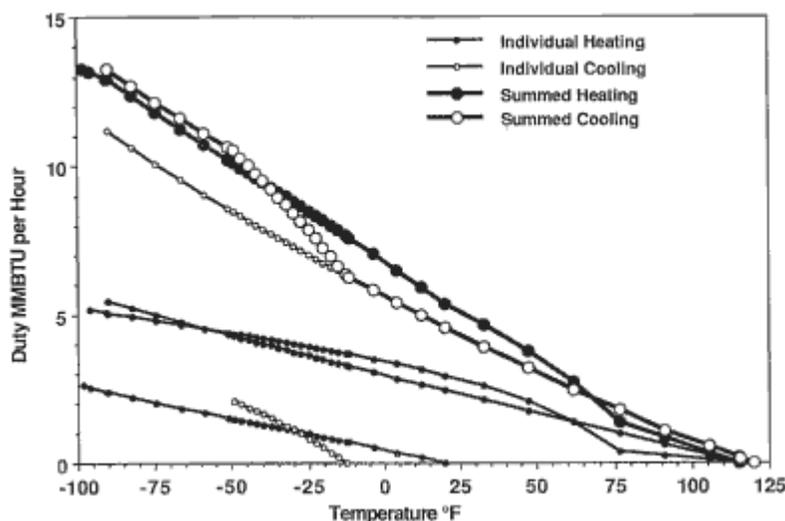
Figure 7. Trial 1: Incremental duties for complex exchanger for ethane recovery unit in Case 2.
