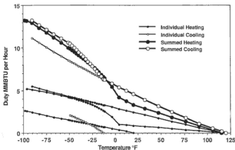
Figure 8. Trial 2: Incremental duties for complex exchanger for ethane recovery unit in Case 2.
