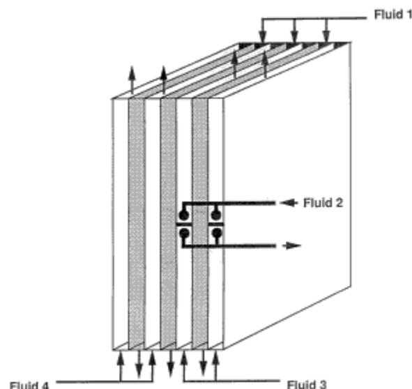
Figure 1. Schematic of complex plate exchanger.
