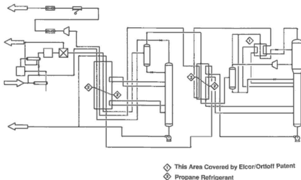
Figure 10. Process flow for liquids recovery from rich gas using refrigeration and expander for Case 3.
