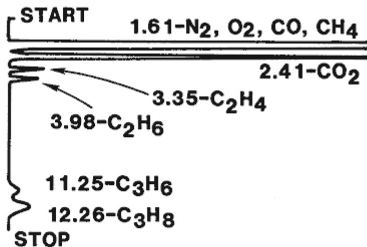
Figure 7. GC results using TENAX-GC and POROPAK Q columns at 80°C.
