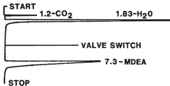
Figure 4. GC results using TENAX-GC and POROPAK Q columns with temperature programming.
