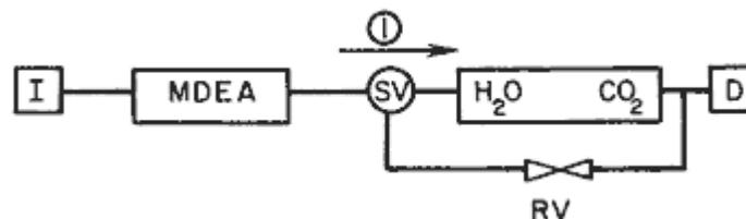
Figure 2. Initial position of GC switching valve.
