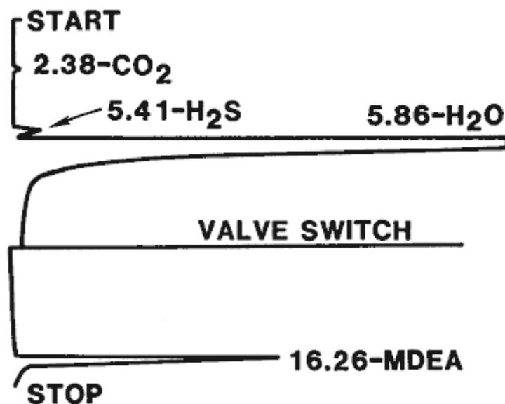
Figure 5. GC results using TENAX-GC and POROPAK Q columns with temperature programming.
