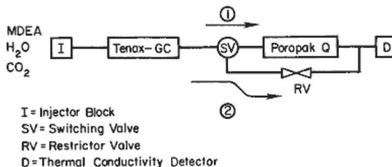
Figure 1. GC column configuration.
