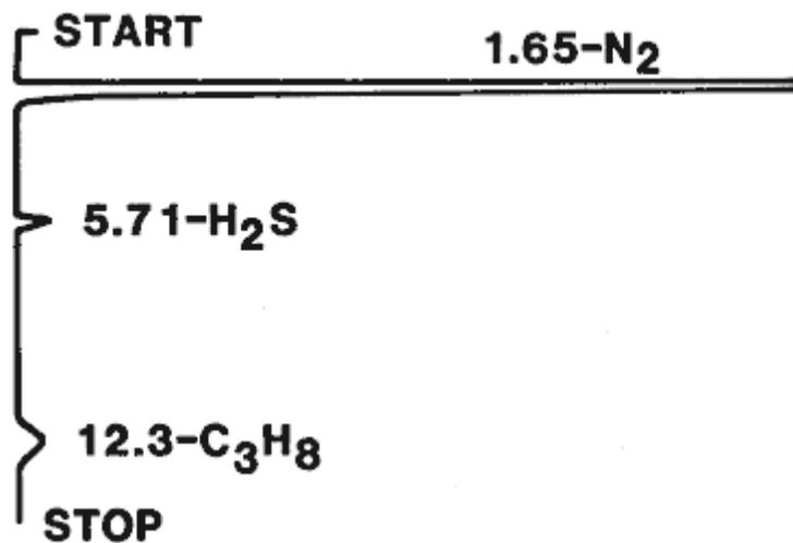
Figure 6. GC results using TENAX-GC and POROPAK Q columns at 80°C.
