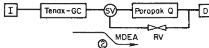
Figure 3. Final position of GC switching valve.
