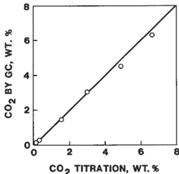
Figure 8. Comparison of analysis for CO<sub>2</sub> in MDEA by gas chromatography and titration.
