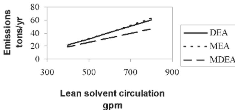
Figure 2. BTEX Emissions vs. Lean Amine Circulation
