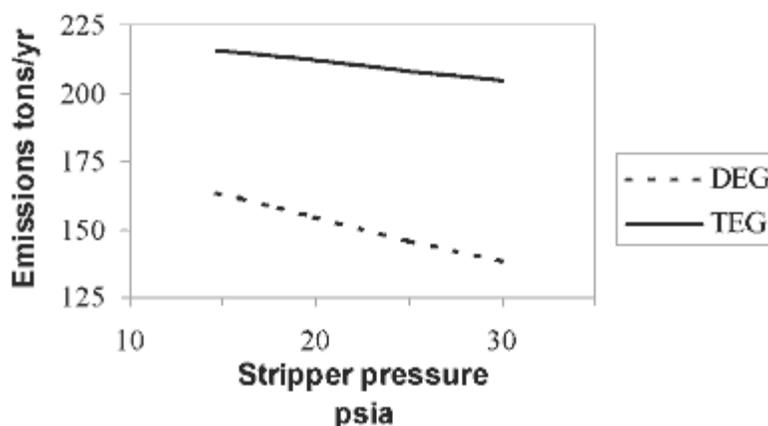
Figure 9. BTEX Emissions vs. Glycol Stripper Pressure
