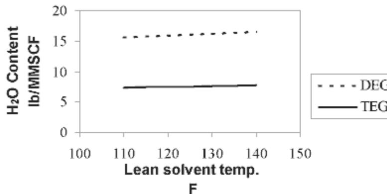
Figure 8 – Residual Water Content vs. Lean Glycol Temperature
