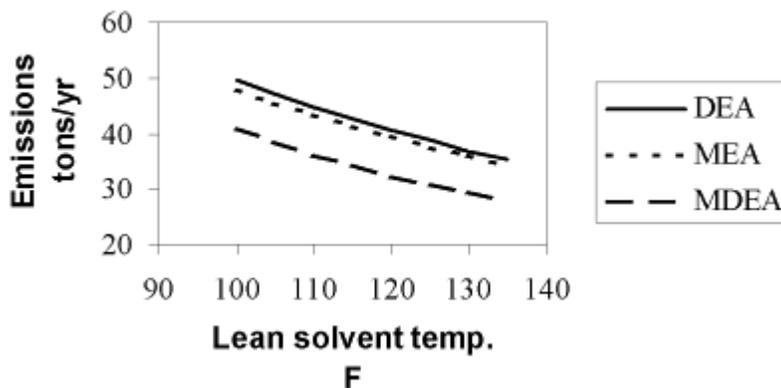
Figure 3. BTEX Emissions vs. Lean Amine Temperature
