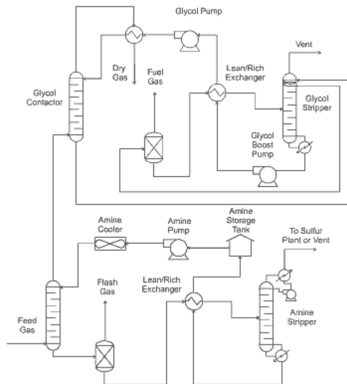
Figure 1. Integrated Gas Processing Plant
