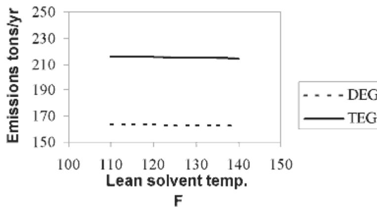
Figure 7. BTEX Emissions vs. Lean Glycol Temperature
