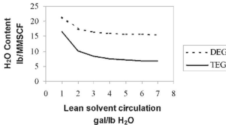
Figure 6. Residual Water Content vs. Lean Glycol Circulation
