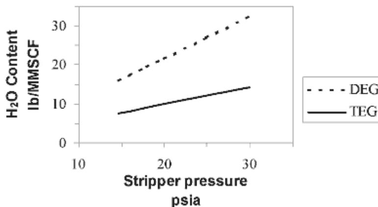
Figure 10. Residual Water Content vs. Glycol Stripper Pressure
