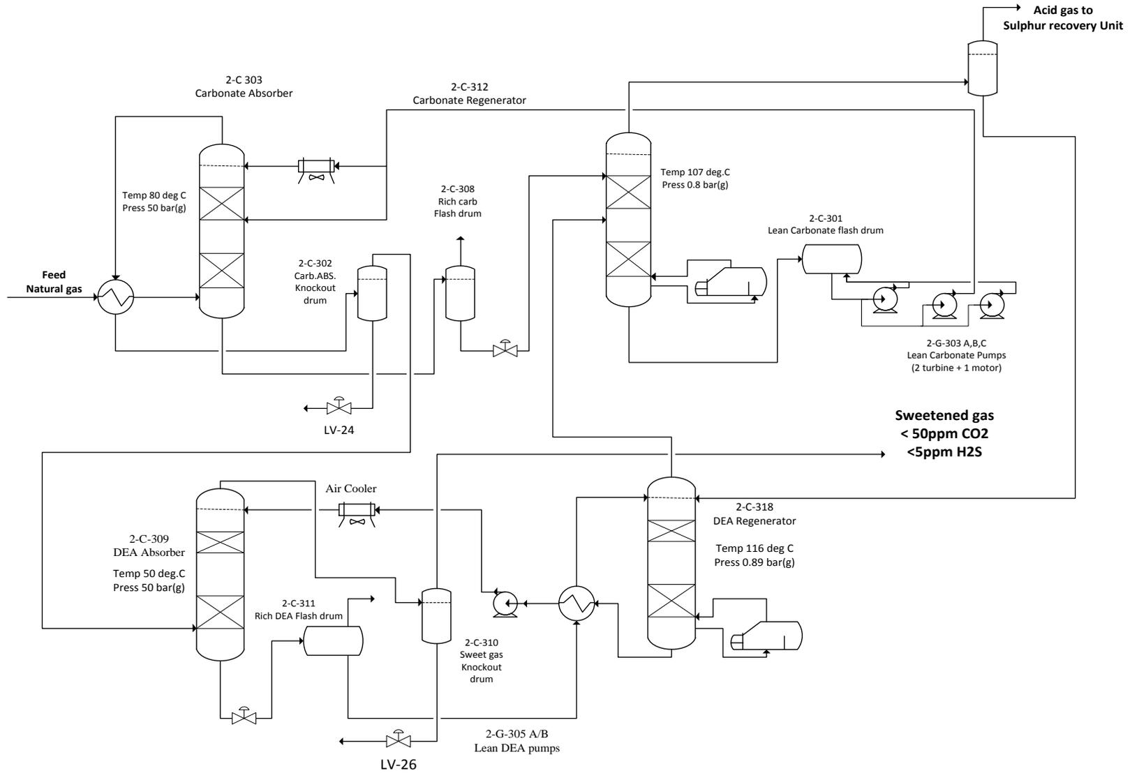
**Figure 1:** ADGAS' Train#3 gas treating plant – Schematic of the Benfield HiPure process
