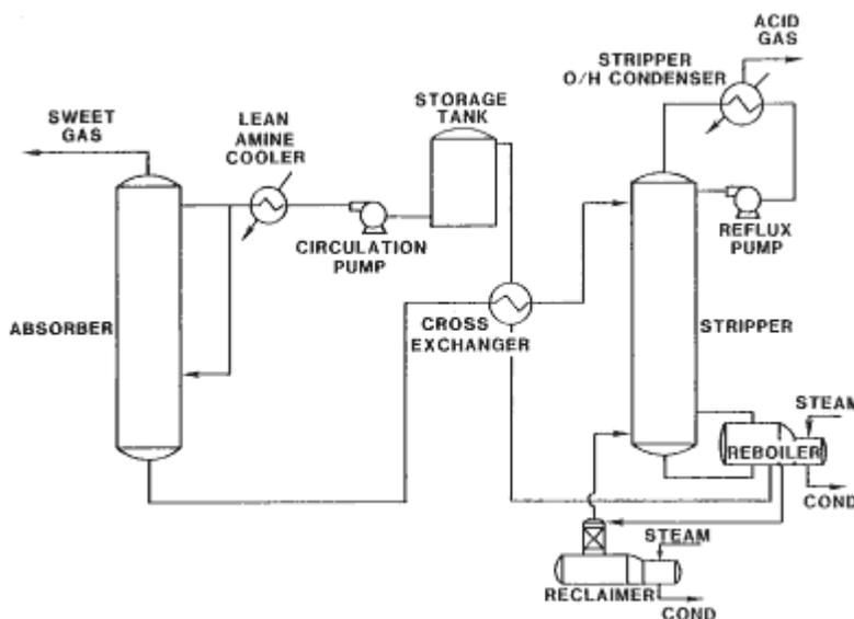
Figure 2. Process flow sheet for multiple feed absorber.
