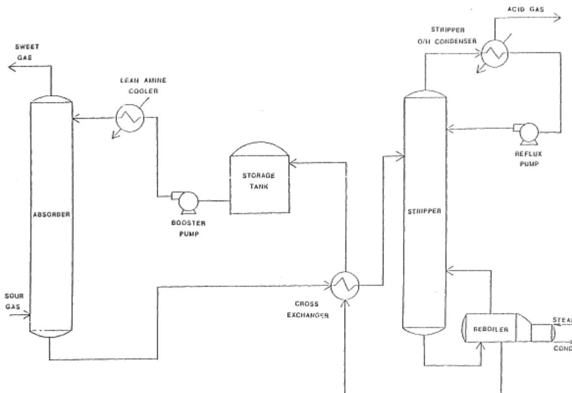
Figure 1. Process flow sheet for common sweetening plant.
