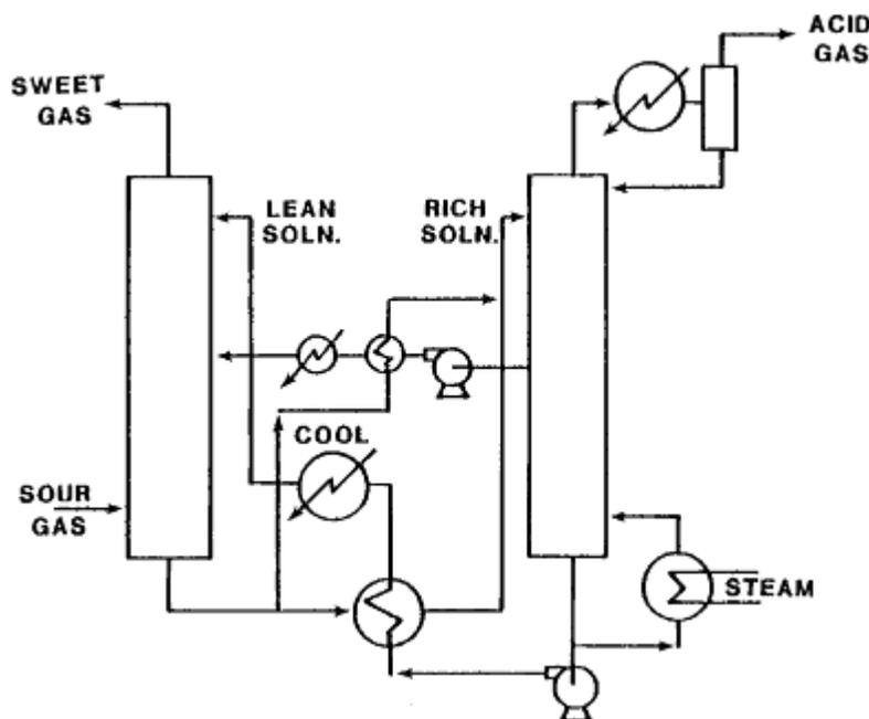
Figure 5. Flow sheet for split flow plant.
