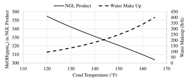
Figure 3: NGL Methanol Content and Water Makeup vs. Condenser Temperature
