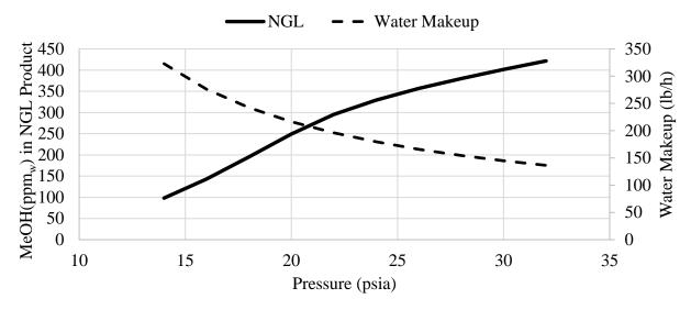
Figure 6: Stripper Pressure Impact on Methanol in the NGL and Water Makeup
