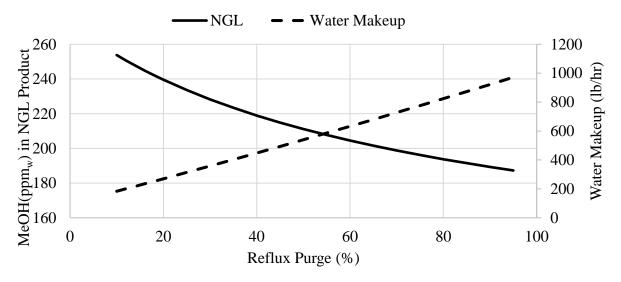
Figure 7: Reflux Purge Effect on Methanol in the NGL and Water Makeup
