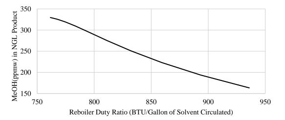
Figure 5: NGL Methanol Content vs. Reboiler Duty Ratio at 70 sgpm Solvent Circulation Rate and 140 °F Condenser Temperature
