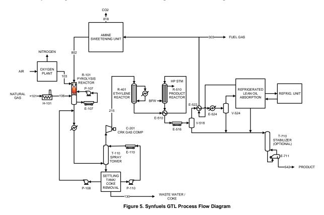
The residue gas is available for use as fuel. To reduce the buildup of inerts in the recycle loop, an Amine Sweetening Unit removes the carbon dioxide from the fuel gas returning to the burner. The remainder of the fuel is available for heating or power production.
