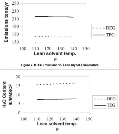
Figure 8 – Residual Water Content vs. Lean Glycol Temperature
