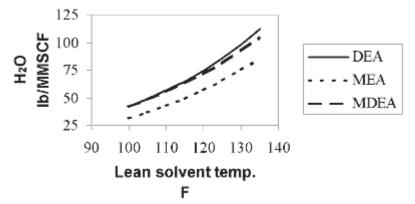
Figure 4. Water in Sweetened Gas vs. Lean Amine Temperature
