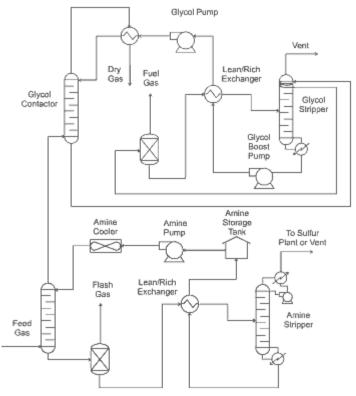
Figure 1. Integrated Gas Processing Plant
