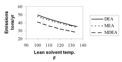
Figure 3. BTEX Emissions vs. Lean Amine Temperature
