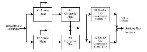
Figure 1 – Plant "A" Block Flow
