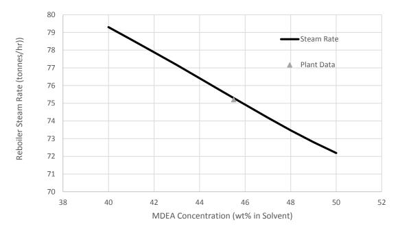
Figure 4: The Effect MDEA Concentration has on the Reboiler Steam Consumption Rate
