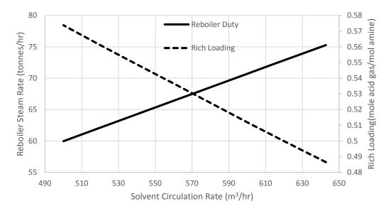
Figure 3: The Impact of Solvent Circulation Rate on the Reboiler Steam Consumption and Rich Loading
