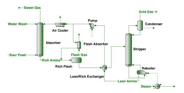
Figure 1: Typical GASCO MDEA Sweetening Unit
